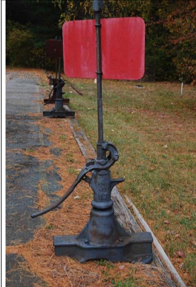
Switchstands. Near and center are B&MRR. Stand in distance is typical of period but not from this railroad.
