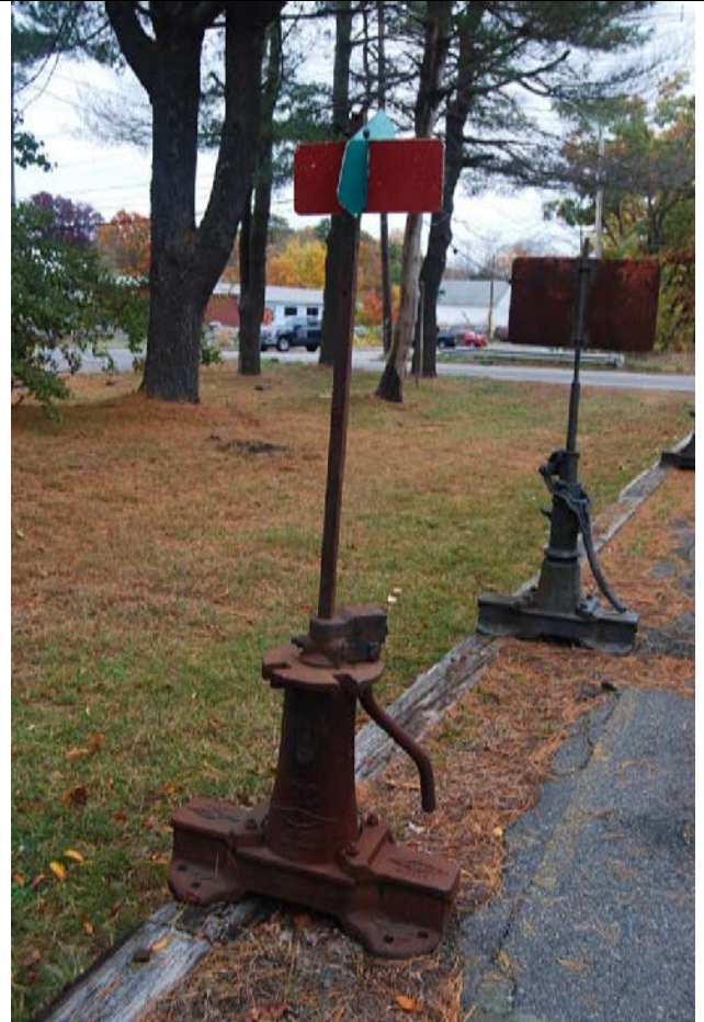
Switchstands. Center stand is B&MRR Ramapo-Ajax Stand No. 17. Stand in foreground is typical of period but not from this railroad.
