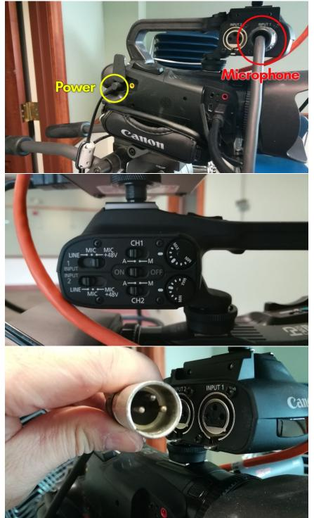
a. INPUT 1: MIC +48V-----CH1: A-----SWITCH ON
