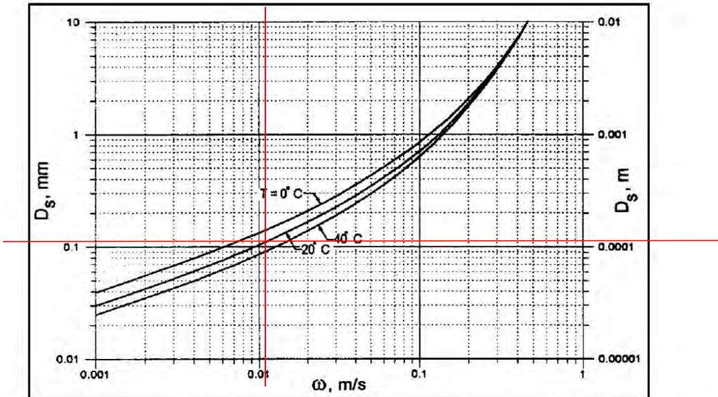
Figure 6.8. Fall velocity of sand-sized particles with specific gravity of 2.65 in metric units.
