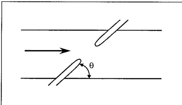
Figure 7.5. Orientation of embankment angle,  $\theta$ , to the flow.
