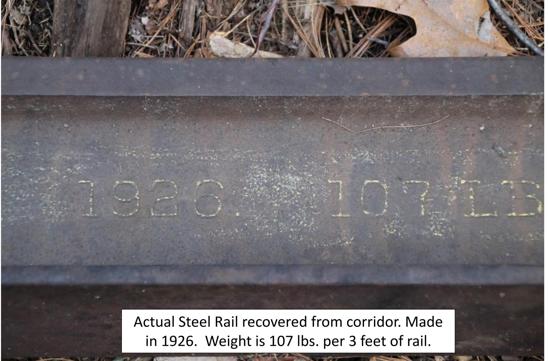
Actual Steel Rail recovered from corridor. Made in 1926. Weight is 107 lbs. per 3 feet of rail.
